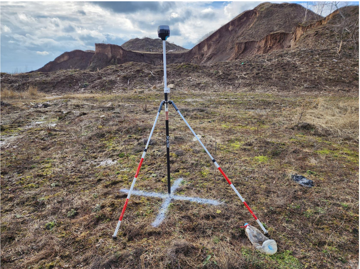
Reach RS2 receiver operating in base station mode.
