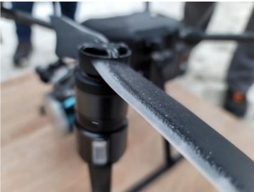
Icing of the drone during flight at -18^{\circ}\text{C} propeller
