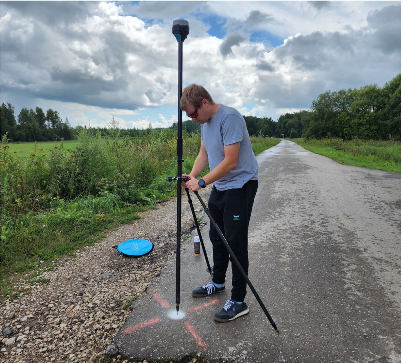
A ground control point made with paint on the pavement is coordinated using the Reach RS2 GNSS receiver.
