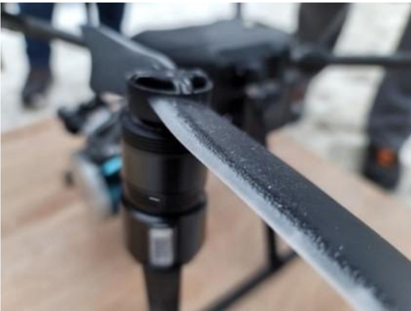
Icing of the drone during flight at -18^{\circ}\text{C} M200 propeller
